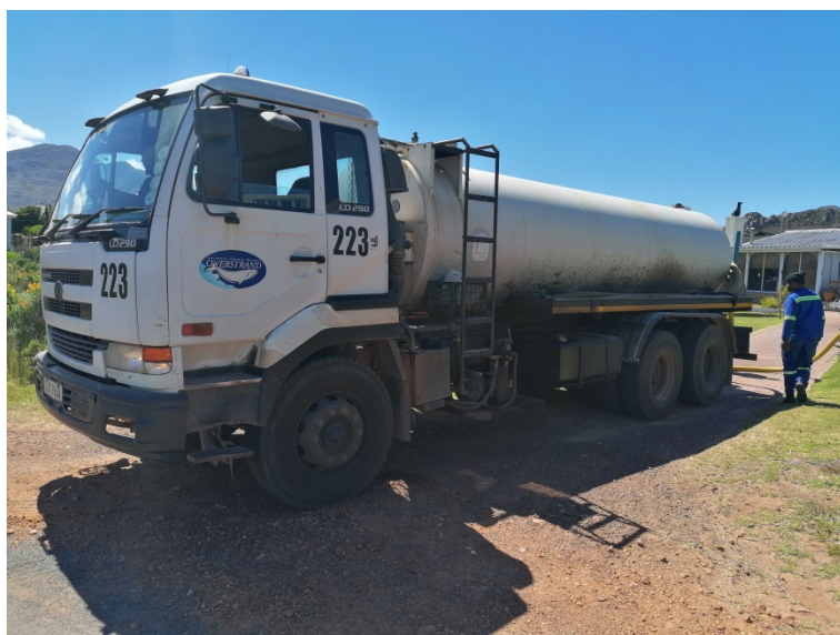
Municipal vacuum tanker emptying a conservancy tank
